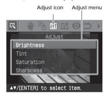
3 Press △/▽ to select the desired adjustment tool and press ENTER. The adjustment slider appears.
